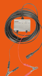
BCL52CNV 36 V to 12 V convertor
